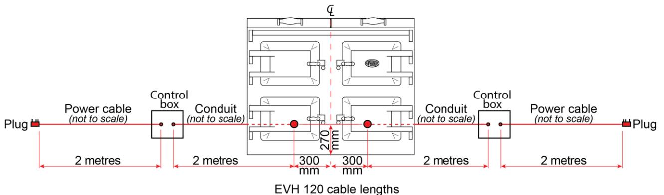
The control boxes should be placed one immediately either side of the cooker to ensure sufficient length of conduit for installation, each adjacent to a 13 Amp socket. If this is not possible, please contact Everhot for further information.
